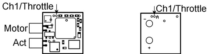
3-6v may be connected with correct orientation to +/- magnets/pads under the board.
