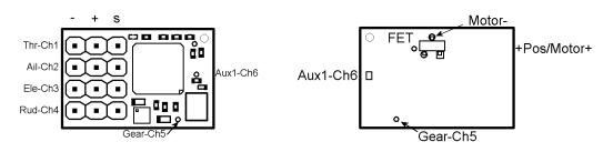
3-6v may be connected with correct orientation to +/- pads. Ch1-4 pads marked 's', Ch5 and Ch6 are signal connections. The Rx is not insulated so take care to avoid short circuits. The PCB is thin so do not bend it or exert great force on it. The receiver will work with DSM2-capable transmitters (surface and air). The Tx/Rx may be switched On/Off in any order.
